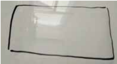
Scratch resistance glass after cycling friction movement
